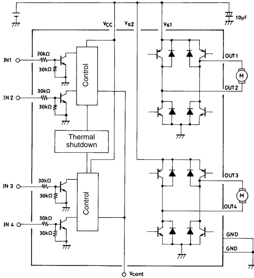
Note: As long as the voltages applied to  $V_{CC}$ ,  $V_{S1}$ ,  $V_{S2}$ , and  $IN1$  through  $IN4$  are within the limits set by the absolute maximum ratings, there are no restrictions on the relationship of each voltage level in comparison with the others (regarding which is higher or lower). (ex.  $V_{CC} = 3\text{ V}$ ,  $V_{S1, 2} = 2\text{ V}$ ,  $IN1$  to  $IN4 = 5\text{ V}$ )
