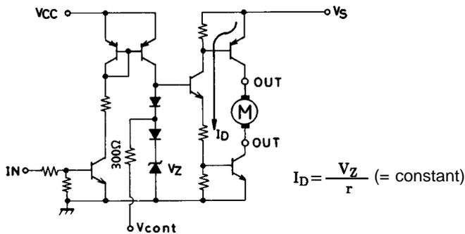
As shown in the above diagram, the  $V_{cont}$  pin outputs the voltage of the band gap Zener  $V_Z + V_F (= 1.93\text{ V})$ .
