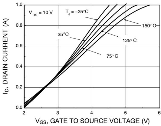
Figure 5. Transfer Characteristics
