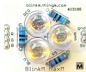
Photo 1.3.2: BlinkM MaxM "Blaster"
