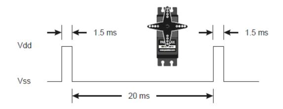
As the length of the pulse decreases from 1.5 ms, the servo will gradually rotate faster in the clockwise direction, as can be seen in the figure below:
