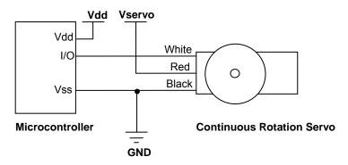
Vdd = microcontroller voltage supply
