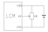
VDD~V0: LCD Driving voltage
