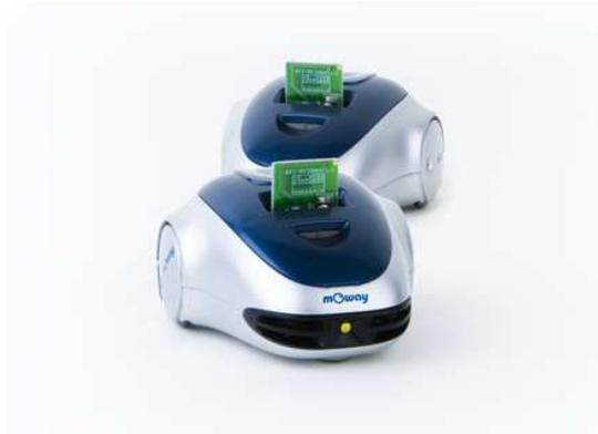
Image 12. RF modules into expansion connector.
