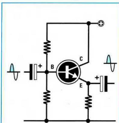
Fig.452 Common Collector.
