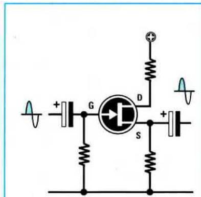
Fig.508 Common Drain
