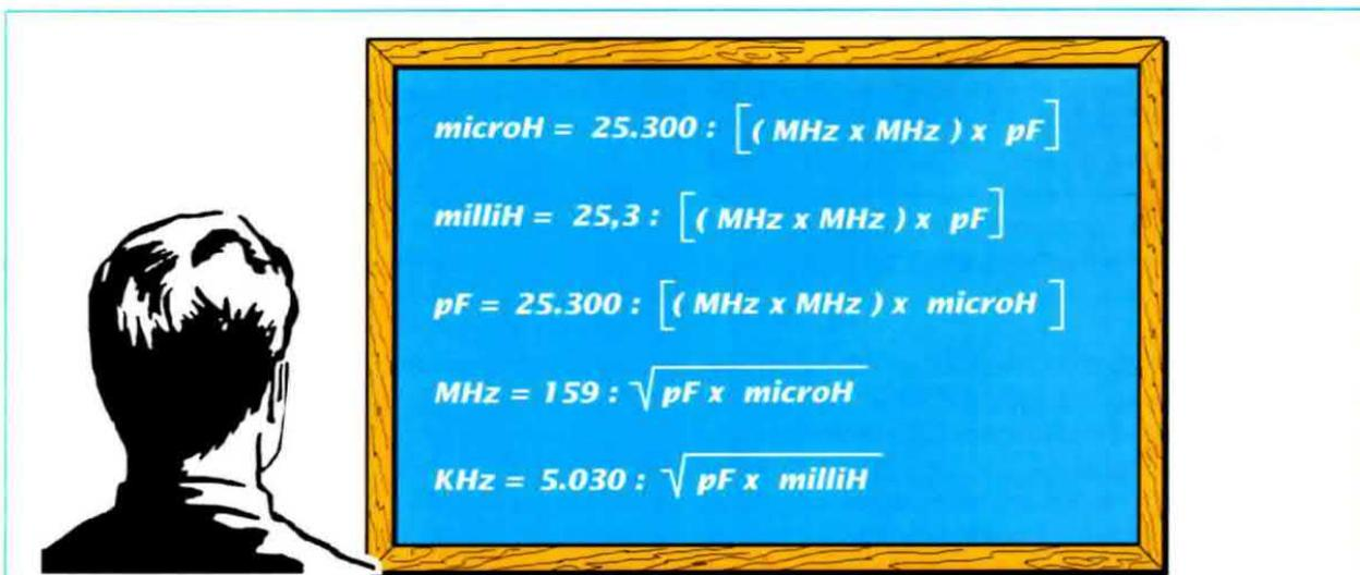
$$\text{microH} = 25.300 : [ (\text{MHz} \times \text{MHz}) \times \text{pF} ]$$
