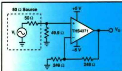
Output Voltage Noise Density of 6.8 nV/√Hz
