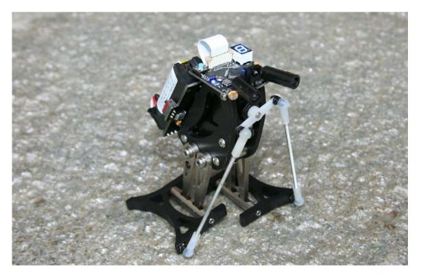
The Penguin's microcontroller is an embedded BASIC Stamp2px24 module, the fastest and most powerful BASIC Stamp microcontroller model in the Parallax lineup. The Penguin requires three hours to assemble, after which it is a PBASIC programming challenge to exploit all of the robot's capabilities.
