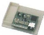
LA SCHEDA CPU CON LA SD CARD INSERITA SUL SUPPORTO E ASSEMBLATE NELL'USCITA 44
