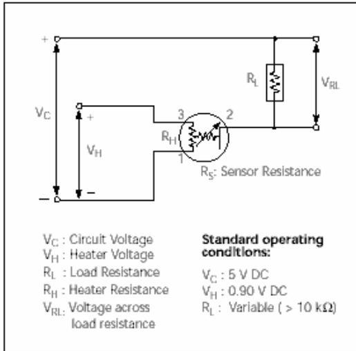
Fig 2. Standard circuit
