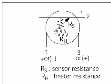
**Fig 1c. Equivalent circuit**
