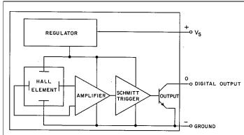
Figure 2-12 NPN (Current sinking) . . . Digital output sensor
