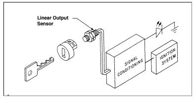
Figure 7-12 Door interlock sensor
