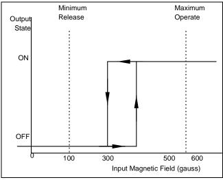
Figure 2-13 Unipolar input characteristics . . . Digital output sensor
