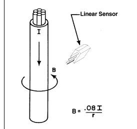
Figure 7-21 Simple current sensor
