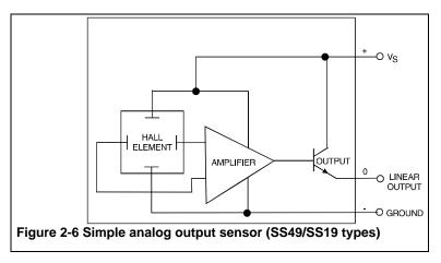
To further increase the interface flexibility of the device, an open emitter, open collector, or push-pull transistor is added to the output of the differential amplifier. Figure 2-6 shows a complete analog output Hall effect sensor incorporating all of the previously discussed circuit functions.
