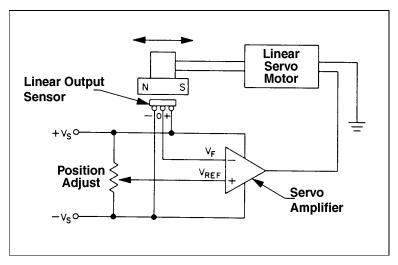
Figure 7-8 Linear feedback sensor for analog control systems
