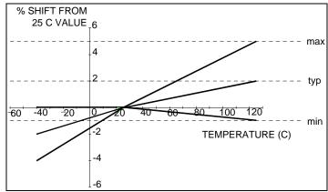
Figure 2-9 Sensitivity shift versus temperature
