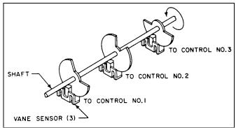
Figure 7-2A Cam-operated vane sensors
