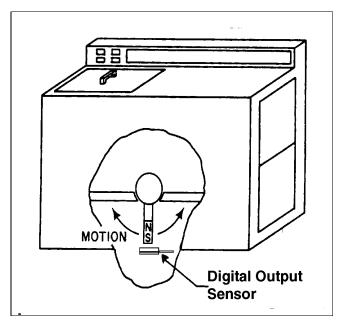
Figure 7-16 Level/tilt sensor
