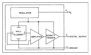
Figure 2-10 Digital output Hall effect sensor
