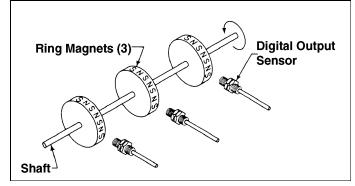
Figure 7-2B Ring magnet operated sensors
