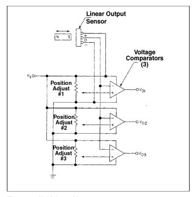
Figure 7-9 Multiple position sensor
