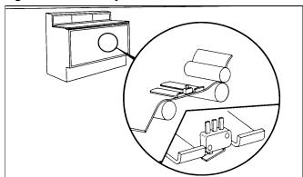
Figure 7-4 Paper detection sensor
