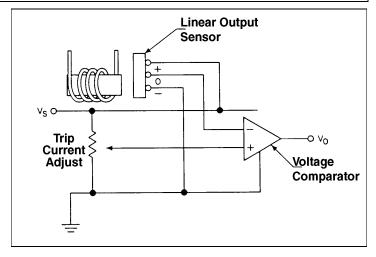
Figure 7-7 Adjustable current sensor
