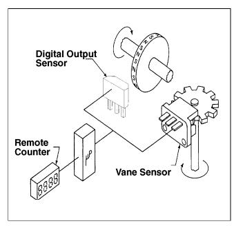
Figure 7-20 Remote reading sensor
