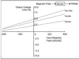
Figure 2-8 Transfer function . . . Analog output sensor
