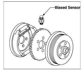
Figure 7-11 Anti-skid sensor
