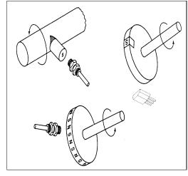
Figure 7-18 Basic RPM sensors
