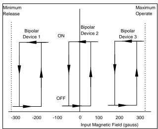
Figure 2-14 Bipolar input characteristics . . . Digital output sensor
