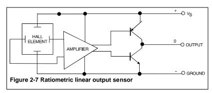
Figure 2-7 illustrates a ratiometric analog sensor that accepts a 4.5 to 10.5 V supply. This sensor has a sensitivity (mV/Gauss) and offset (V) proportional (ratiometric) to the supply voltage. This device has "rail-to-rail" operation. That is, its output varies from almost zero (0.2 V typical) to almost the supply voltage (Vs - 0.2 V typical).
