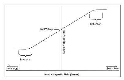
Figure 2-5 Null voltage concept
