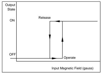
Figure 2-11 Transfer function hysteresis . . . Digital output sensor
