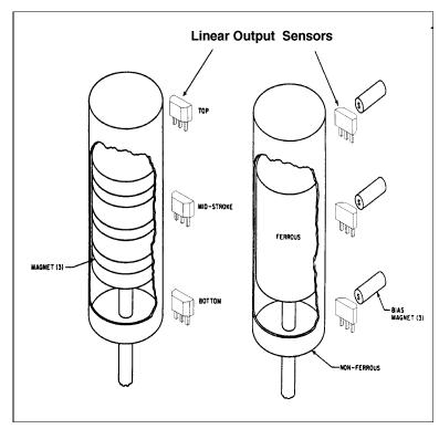
Figure 7-24 Piston detector sensors
