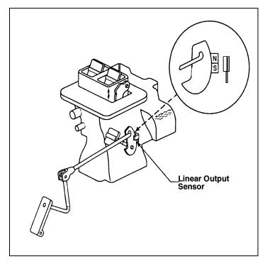
Figure 7-27 Throttle angle sensor
