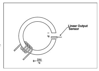
Figure 7-22 Low level current sensor
