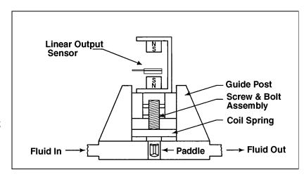
Figure 7-23 Flow rate sensor
