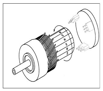
Figure 7-17 Brushless DC motor sensors
